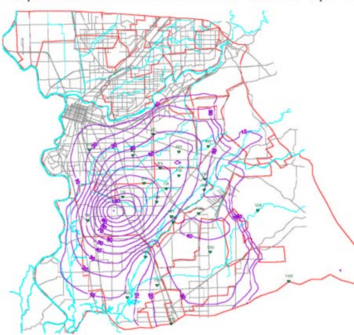
Figure A7: Scenario 3 Groundwater Contour Map – Difference between Scenario 3 and No Action Alternative
